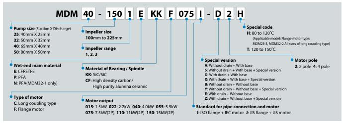
Note: Long coupling type is designed for 50 cycle area.
