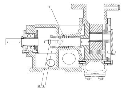
2.7 In case of pumps with packing seal, tighten up the Pos. 13 packing gland lightly using the screws (Pos. 52) (up to a maximum torque of 10 N) and then loosen them slightly again.
